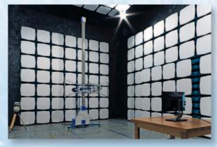
facilitated our chamber with equipment allowing **testing for military purposes**, in accordance with military standards MIL-STD 461F and Polish NO-06-A200 & A500. We can also run a set of immunity tests against temperature (range from -70  $^{\circ}$ C to +180  $^{\circ}$ C), humidity (up to 95%) and mechanical stress (vibrations, single and multiple shocks, user defined shape of pulse).
