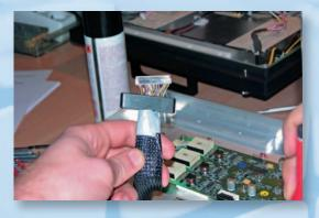
The EMC solution sometimes can be as simple as adding a small shielding, re-routing the wires or adding an ordinary capacitor. But sometimes a more sophisticated EMI filter or even redesign of the PC board is required. We can propose any of the solutions keeping in mind not only EMC compliance, but also cost and long-term production issues.
