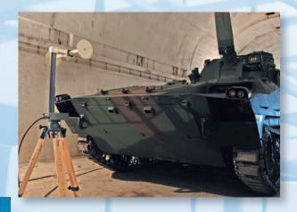
We have committed ourselves into projects concerning products of different scale. For fixed installations and large size mobile objects that are either too big or impractical to be moved into the anechoic chamber, such as military and combat vehicles, we are offering on-site EMC testing package. Our specialist have been thus far arranging and carrying out tests on all sorts of testing grounds, such as OATS, installation sites and other carefully selected locations.
